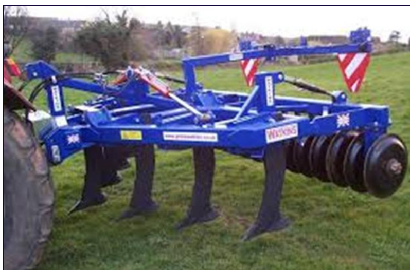
Figure 5.1: Tractor mounted subsoiler
