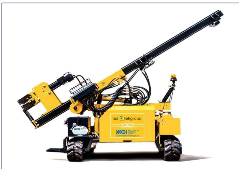
Figure 4.1: Example of a LGP Pile Driver
